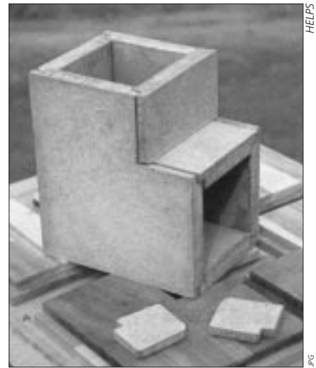
Figure 6: Baldosa tile combustion chamber
