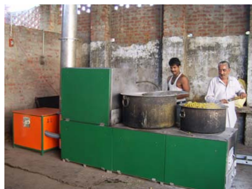
The Sanja Chula in India, cooking meals for school children. It runs on biomass briquettes, has a fan to assist the initial stages of combustion until it is hot and has replaced LPG.
