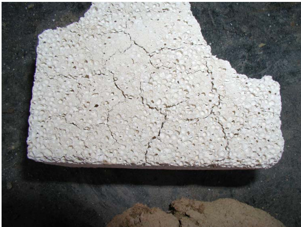
This sample exposed to high temperature developed serious cracking and became weak.
