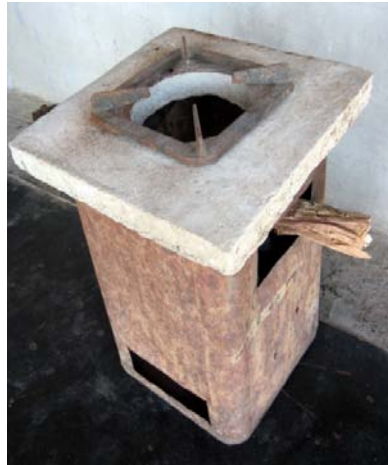
Picture 51 A simple tin stove with a concentrator
