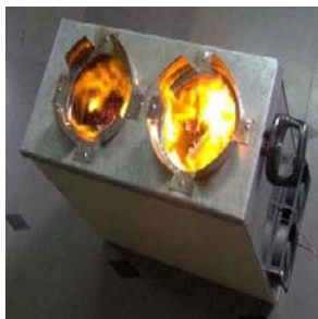
Picture 94 A Computer Processing Unit (CPU) as stove
