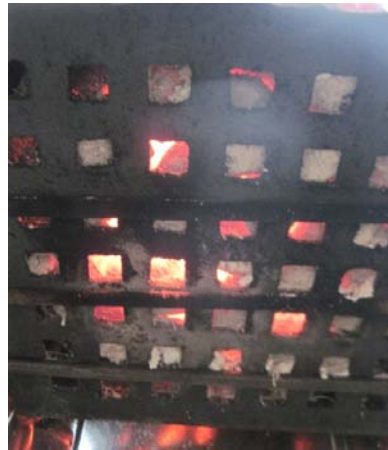
Picture 48 Primary air enters underneath a grate
