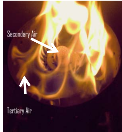
Picture 40 Secondary and Tertiary air
