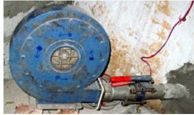
Picture 21 Air blower fitted to a stove, supplies additional air and creates draft for efficient combustion
