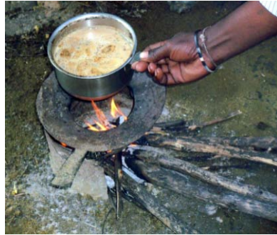
Picture 46 Circular frames made of clay / metal used for prevention of soot on cooking utensils
