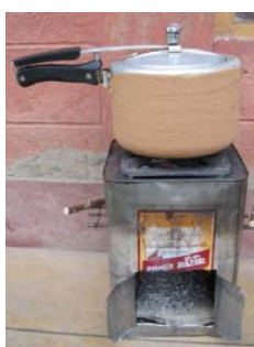
Picture 98 Avani charcoal stove made with used oil tin can
