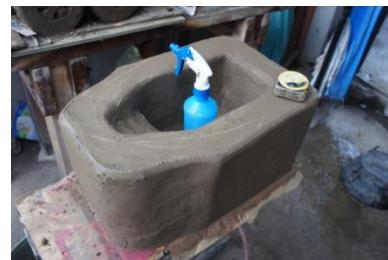
The Holey Roket Stove with a char box as drawn and as built and now drying. Notice the pusher rod (center photo) and the char pocket (upper right photo) on which a can of sardines may fit at the cover and the char box (lower right). Another possible plug would be plaster of paris but should be built only after the stove was fired in the kiln to ensure a tight fit. .
