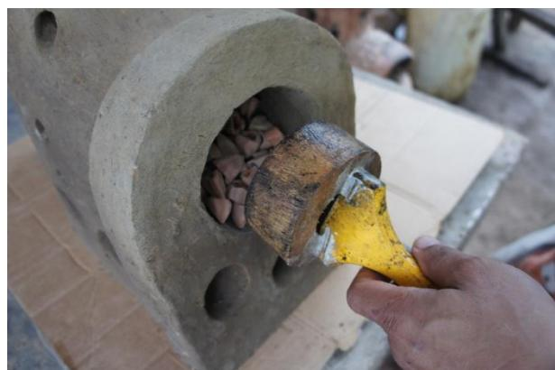
5.5. **Pusher rod for the char.** Unlike the previous pusher rod, this metal rod will push the char into the char pocket.
