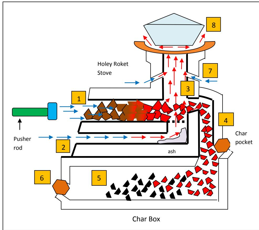
The diagram above illustrates the flow of air, hot gases and char in the stove unit.
