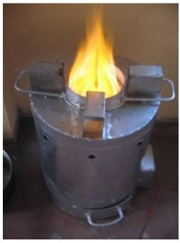
sheet having a diameter of 10 cm and 11 cm, respectively. It is where the pellets are gasified
