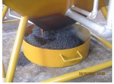
carbonized rice husk as material for composting. It can be fabricated using local materials and skills.
