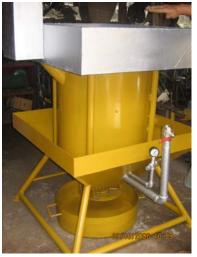
food industry in converting wastes into useful energy. This stove is an offshoot of the R&D on domestic-size rice husk quasi gasifier stove that uses steam injector to improve the burning of gases during cooking. This R&D project on the design and development was assisted by the undergraduate agricultural engineering students Lucio Larano, Daniel Belonio, and Raymond Paul Aungon of the Department of Agricultural Engineering and Environmental Management of the
