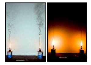
In both pictures biodiesel (left) and kerosene (right) burning in locally made wick-lamps. In the first picture it is possible to see the difference in the amount of smoke emitted. In the second it is possible to see the difference in the intensity of the light (In all the experiments the size o the flame is the same). (Photo Perdomo, Leonardo – TaTEDO, 2006)
