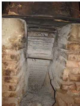
Fig.1.6 : principle of the « stairs feeding » stove used in many small scale productions, mostly for noodle, rice wine and palm sugar.
