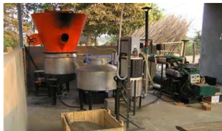
Left: photo of a 7kW power plant (SME project in Battambang). We can notice the red gasifier, the filter on its right and the engine in green, top right.
