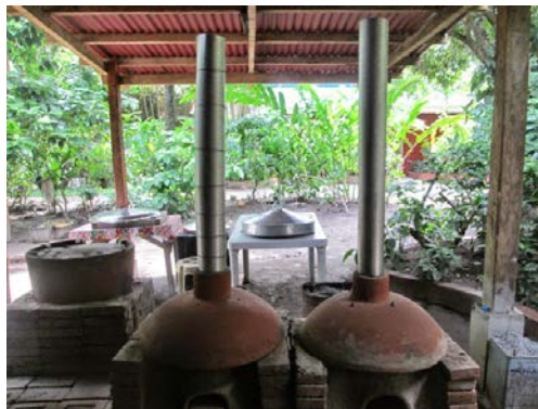
2 DIFFERENT OVEN COVERS FOR CHARCOAL & WOOD FUEL ↑
