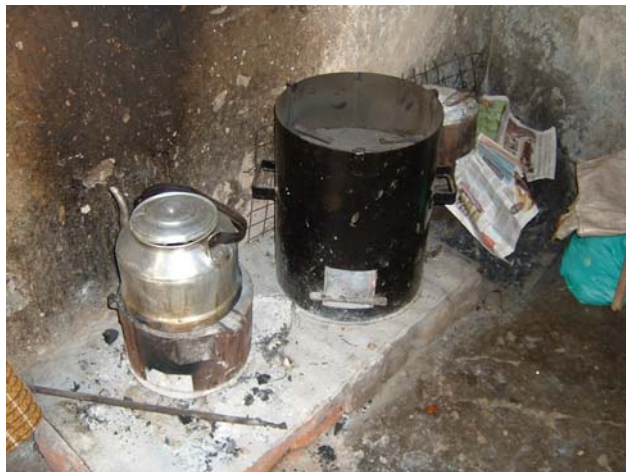
1.9 Four single pot Rocket stoves were produced using Vernacular Insulative Ceramic (VIC) .
