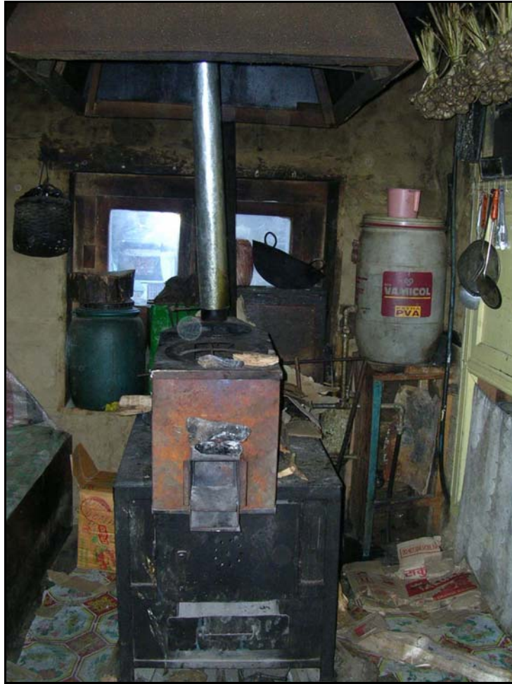
The old metal stove on the bottom weighs about 115 kg and consumes about a Bhari (35 kg) of firewood in one cooking cycle. The new stove (on top) weighs about 20 kg and uses less than 5 kg in one cycle. A plastic barrel on a stand with water heating pipes is on the right-hand side.
