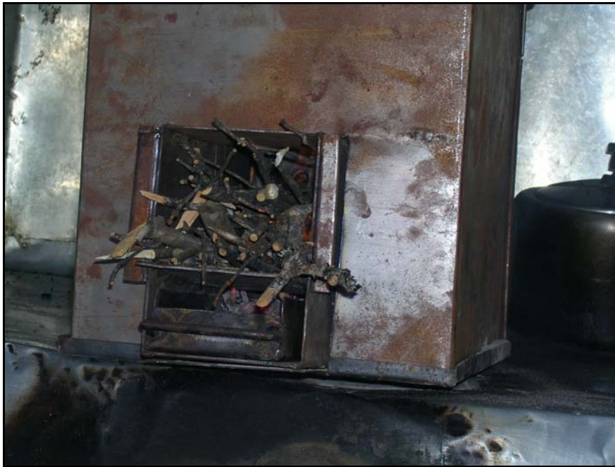
The elbow opening of the new stove is stuffed with small twigs and branches. The metal slide is not inserted here.
