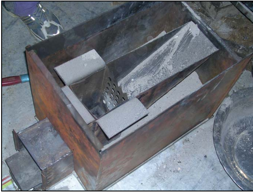
Ashes from the old fireplace are used to insulate the body of the stove. The inner vertical burning chamber can be seen, with holes in the side, allowing the hot flue gasses to lead to the second cooking hole. This inside design will be modified for the next series of stoves.
