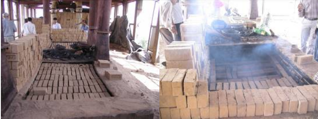
The green bricks are loaded into the shaft from the top.
