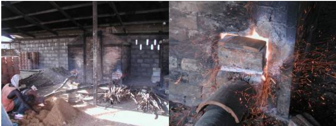
More downdraft kilns in Ghana using sawdust after starting on wood.
