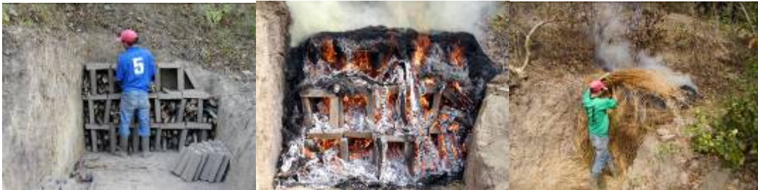
This kiln in El Salvador, while using a massive amount of wood, would probably not be successful without the grass insulation. In addition to adding fuel to the fire, the grass turns to fine ash and retains the heat. About 300 bricks came from this burn.
