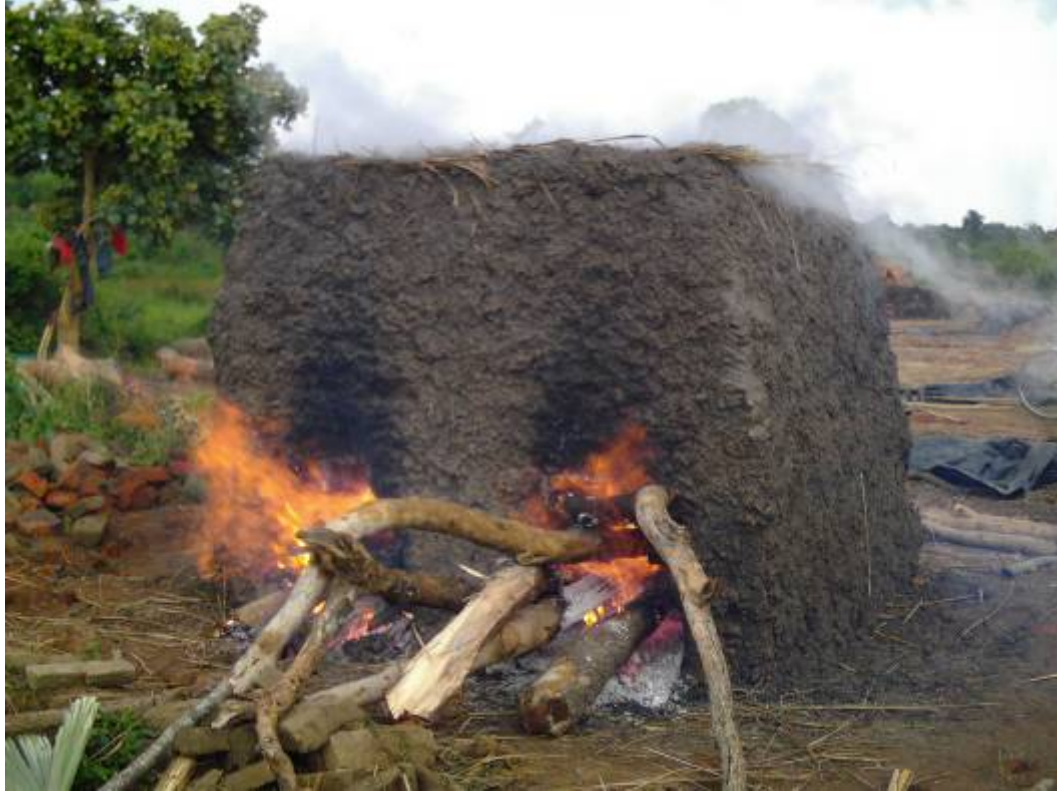
This kiln in Uganda relies on a massive fire but there is some insulation on top. The walls are coated with mud to reduce convection. This kiln contains about 3,000 bricks.
