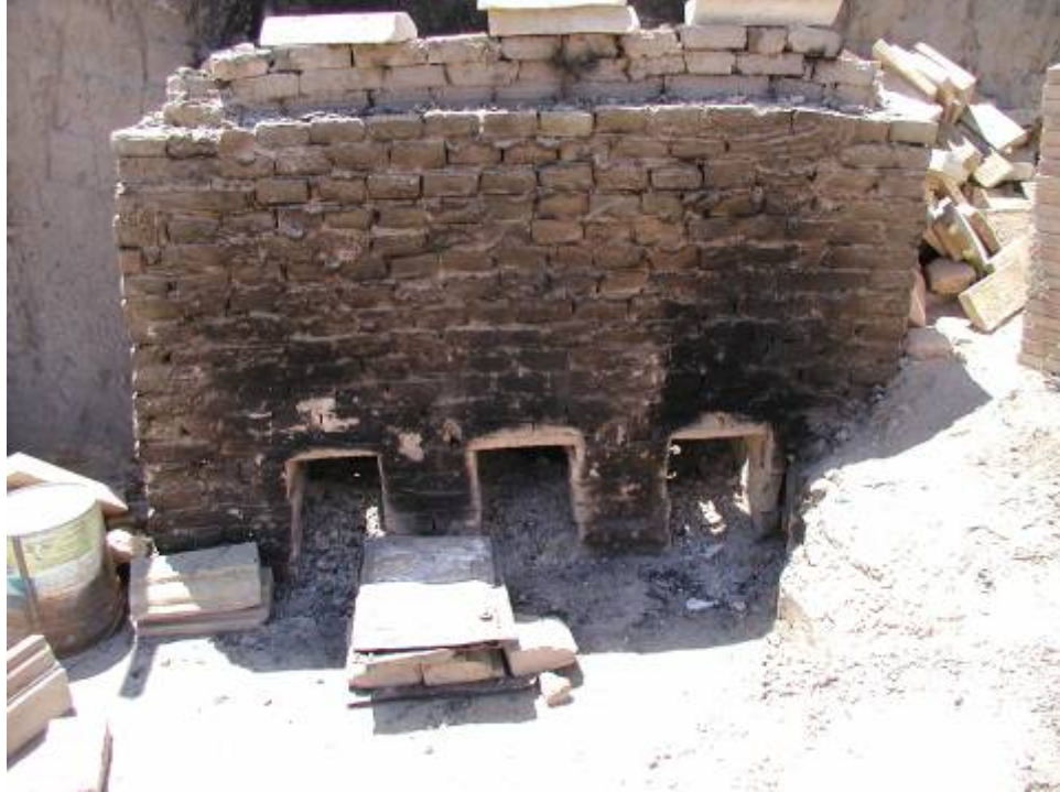
This small kiln in Torreon, Mexico is considered a test kiln. It has no top and maybe grass is placed on top part way through the burn, but maybe not.
