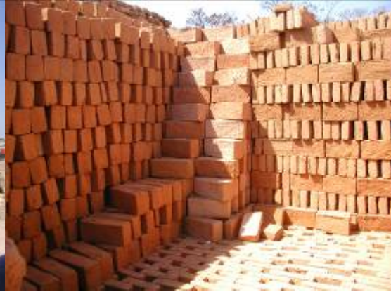
Bricks are stacked in certain patterns to allow heat circulation
