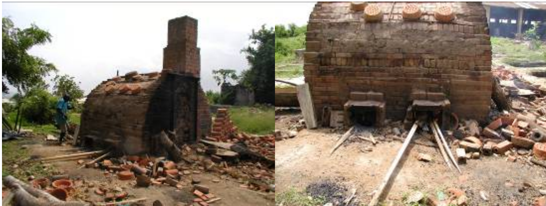
The liners are fired in this down draft kiln.
