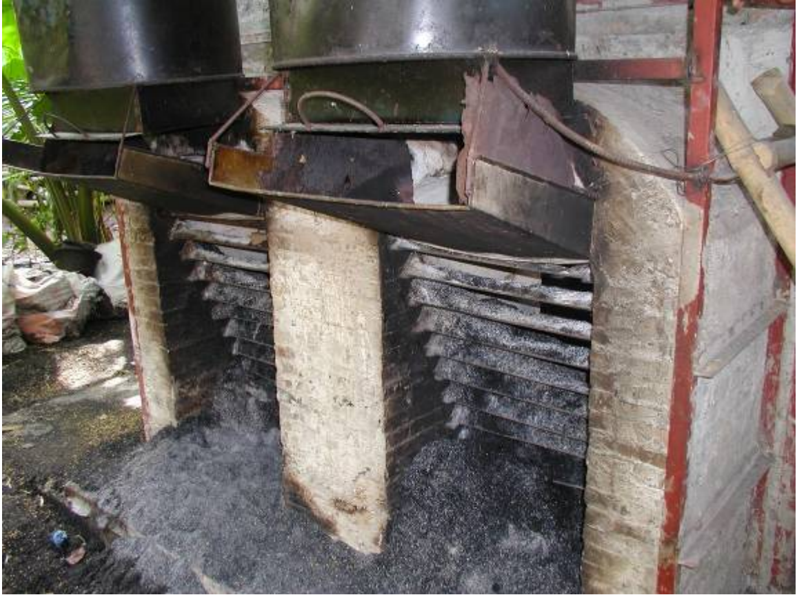
This kiln in the Philippines uses rice husks on a stair step grate for fuel.
