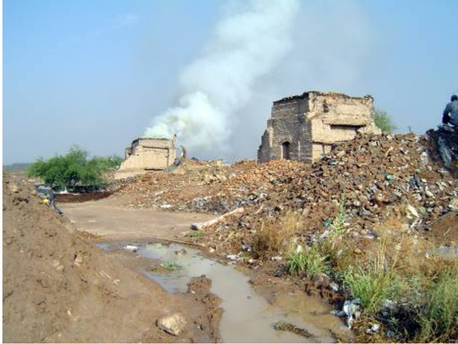
These kilns near Torreon, Mexico fire about 25,000 bricks at once. Since all of the trees and biomass have already been cut down, they now rely on garbage and trash for fuel.
