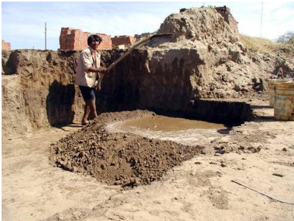
While most brick makers work in teams, Angel, in Salina Cruz, Mexico works by himself. He can make 1,000 bricks per day, but that is unusual (I've never seen anyone work as hard as Angel). He makes bricks to order and fires maybe 5,000 to 7,000 at a time using wood.
