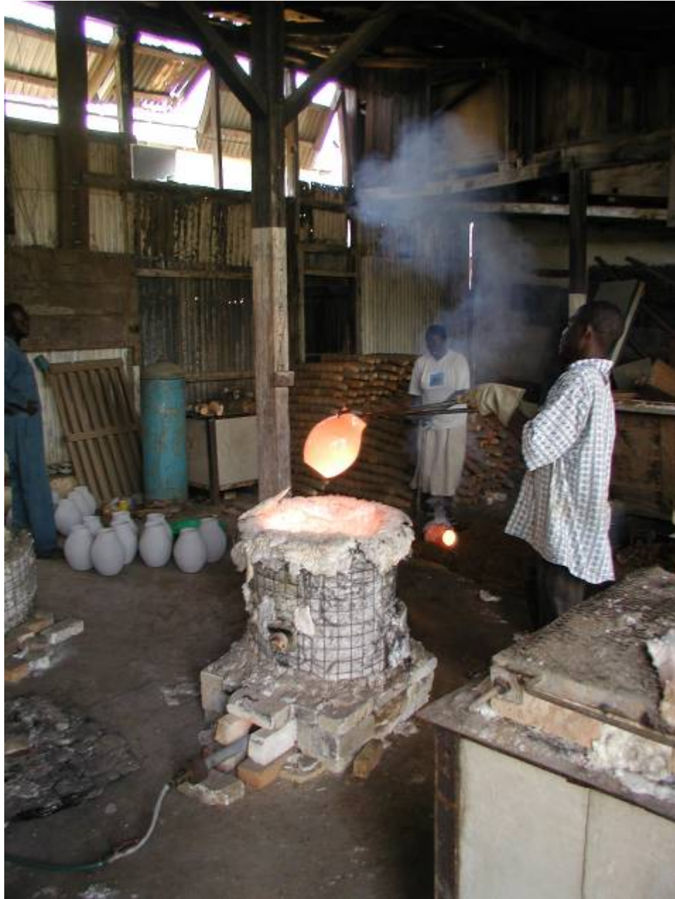
This raku kiln is made from insulating ceramic fiber and is fired with gas.
