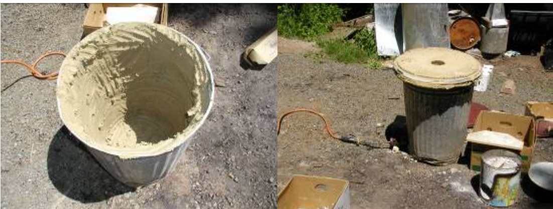
A small gas fired kiln made in a trash can, using a lightweight insulating ceramic mix made from clay and sawdust.
