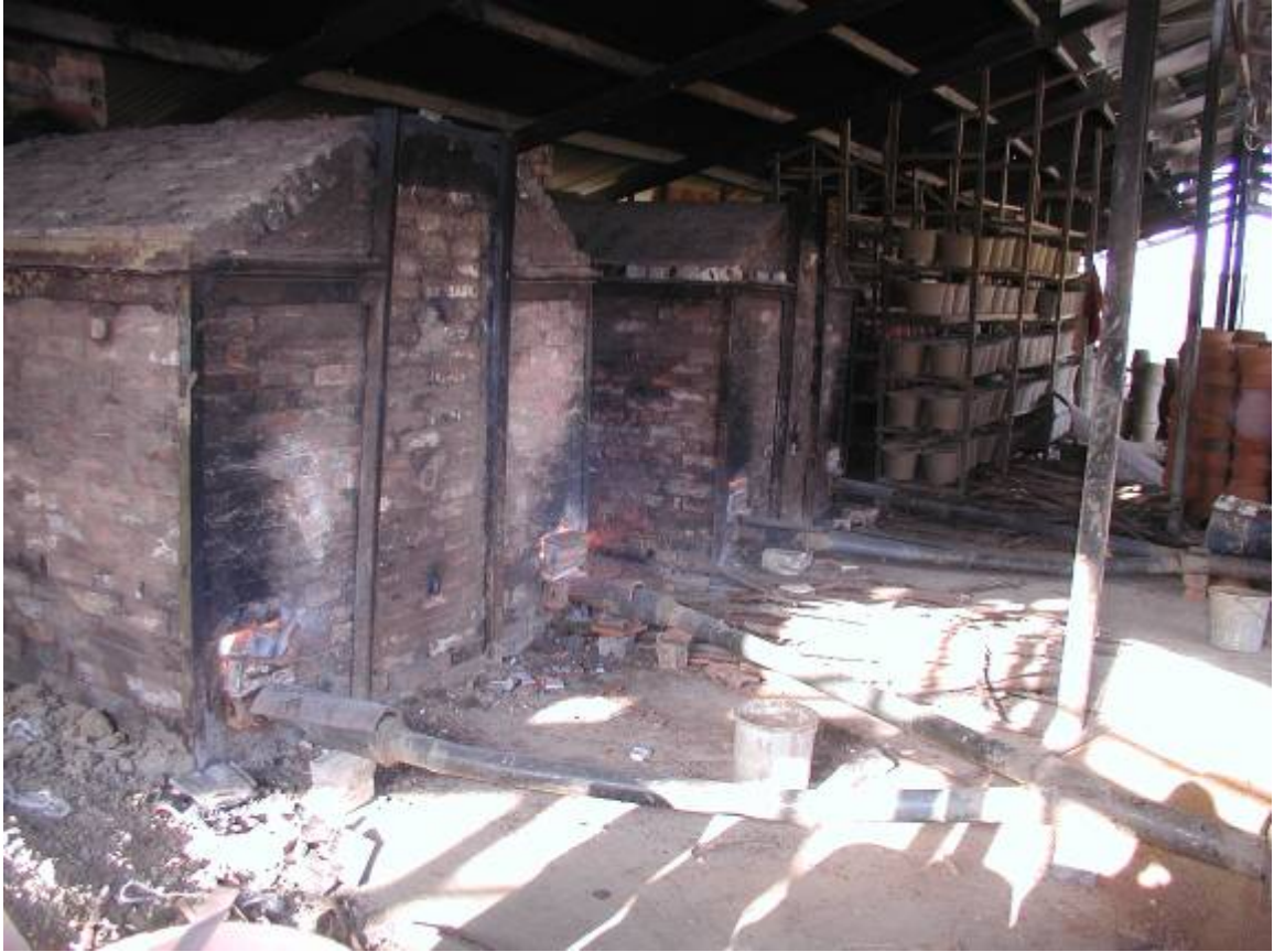
More downdraft kilns in Ghana using sawdust after starting on wood.
