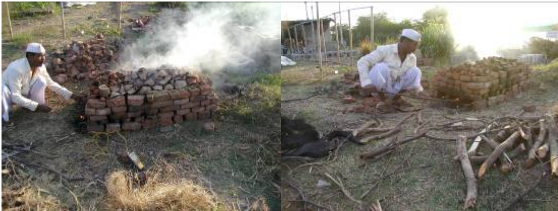
This improvised test kiln in India is being fired using strips of tires for fuel.
