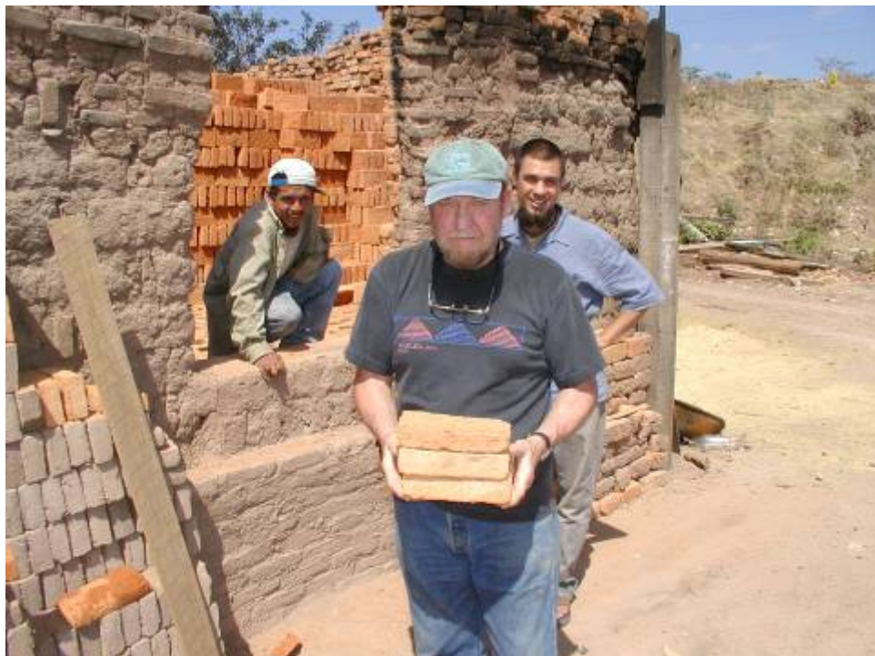
This kiln in Honduras is representative of many kilns in the world. It might have four semi-permanent walls, no roof, wood is placed underneath.
