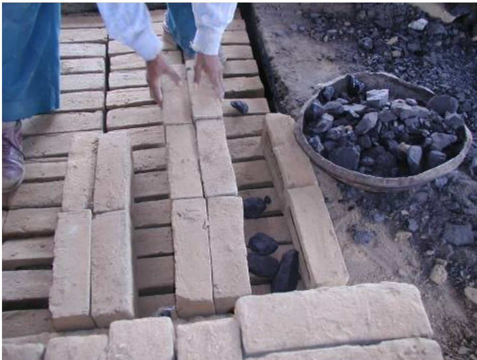
Coal is interspersed with the bricks.
