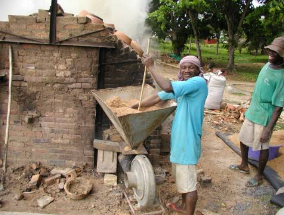
Once the kiln begins to heat up sawdust is blown into the kiln for fuel.
